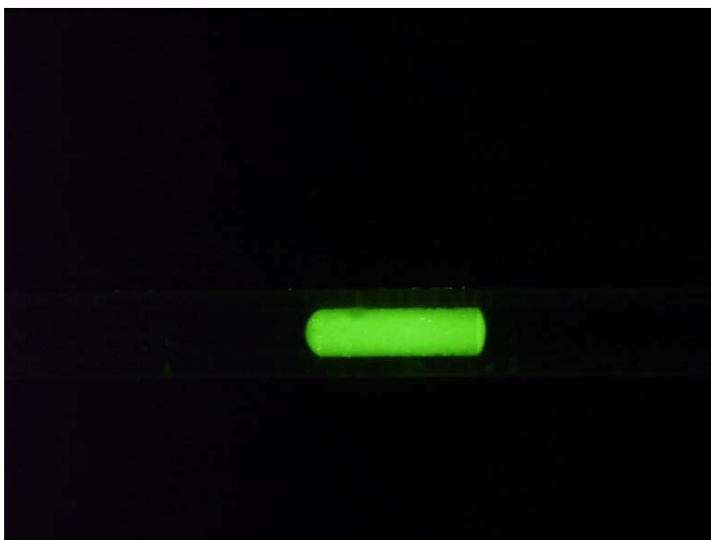
Figure 5: A) (top panel) In an uncoated glass capillary, fluorescent nanospheres are left behind on the capillary wall and also accumulate at the ends of the packet. B) (bottom panel) In a fluorinated capillary, the nanospheres are confined to the packet.
