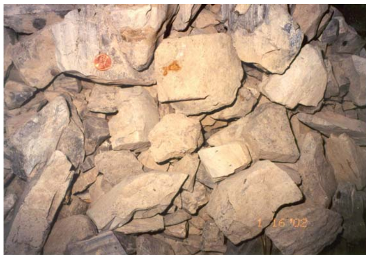
Figure 1. Green River Oil Shale Rubble Collected from the C-A mine site in the Piceance Creek area near Meeker, Colorado.
