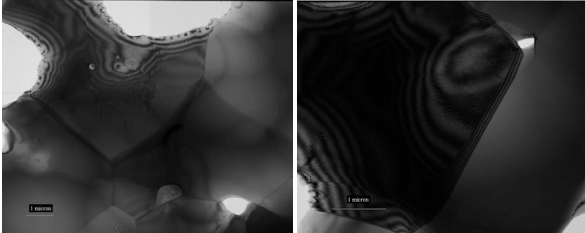
Figure 6.2. TEM images of unirradiated TiN
