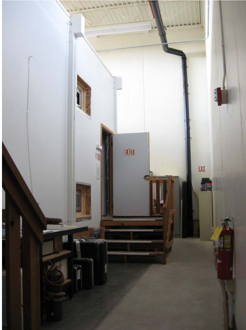
Figure 2. Outside of test room, showing vents and door. The distance between the test room and the building wall is 2.44 m.
