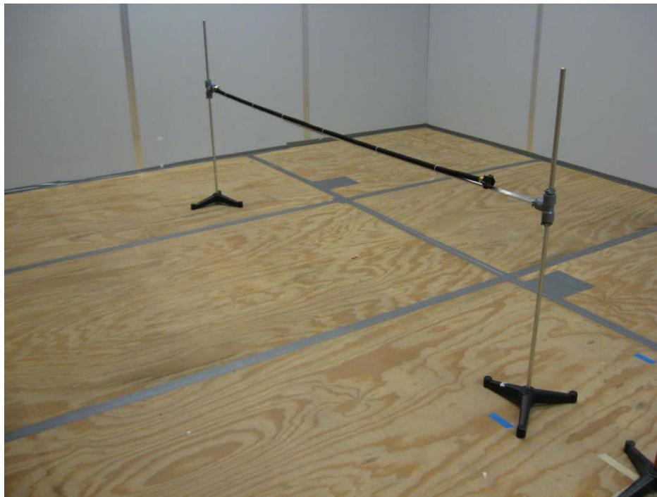
Figure 3. Line diffuser used to inject helium in Cases L1 and L2
