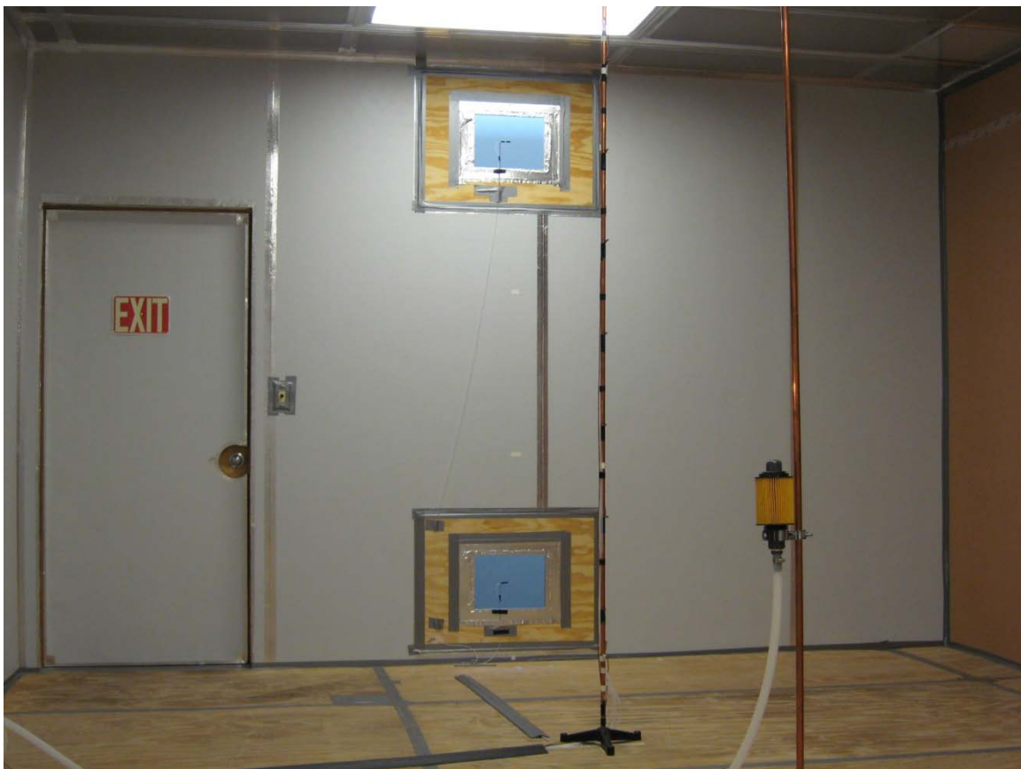
Figure 1. Inside of test room, showing point diffuser, sampling column, vents, and door
