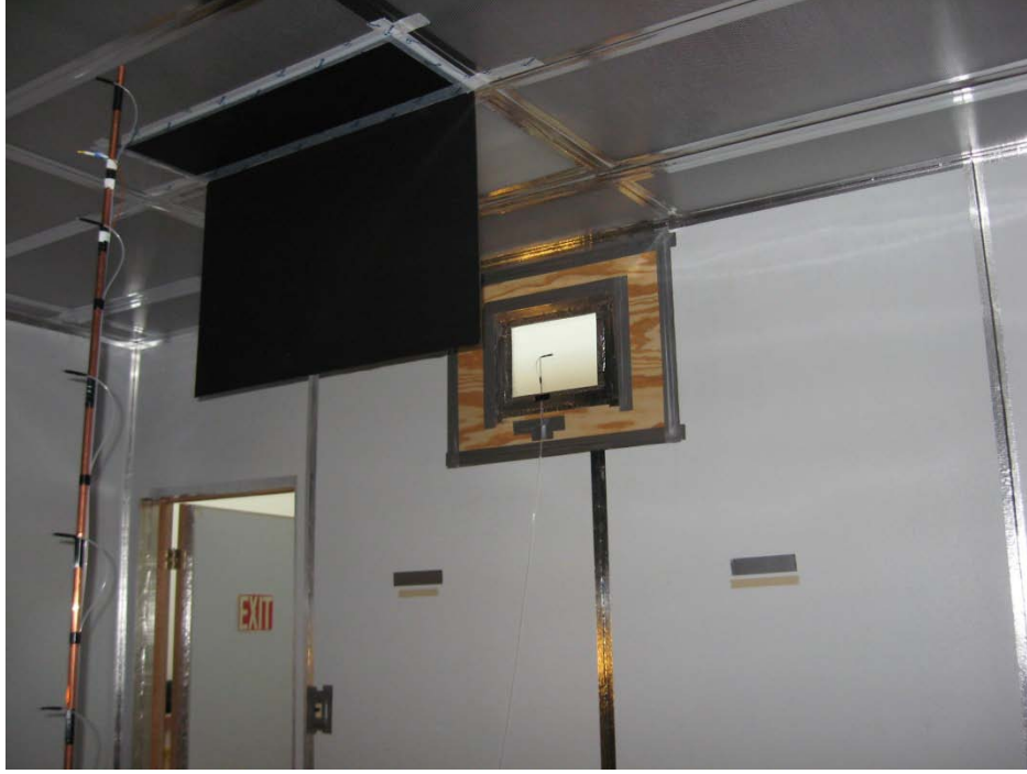
Figure 8. Vent baffle used to test momentum effect in Case P2b
