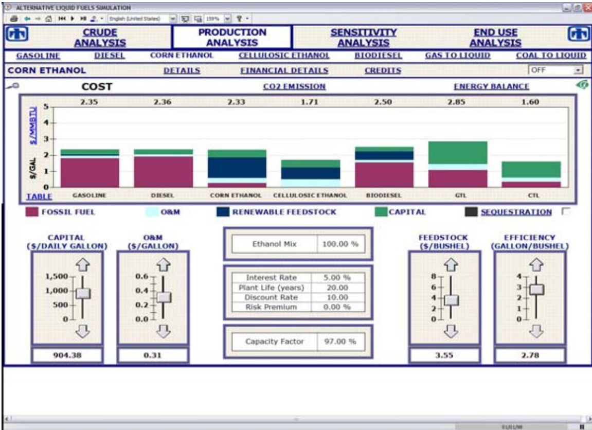
Figure 2. Representative AltSim Production Analysis Screen (corn ethanol) Showing Production Costs for all Fuels by $/gallon
