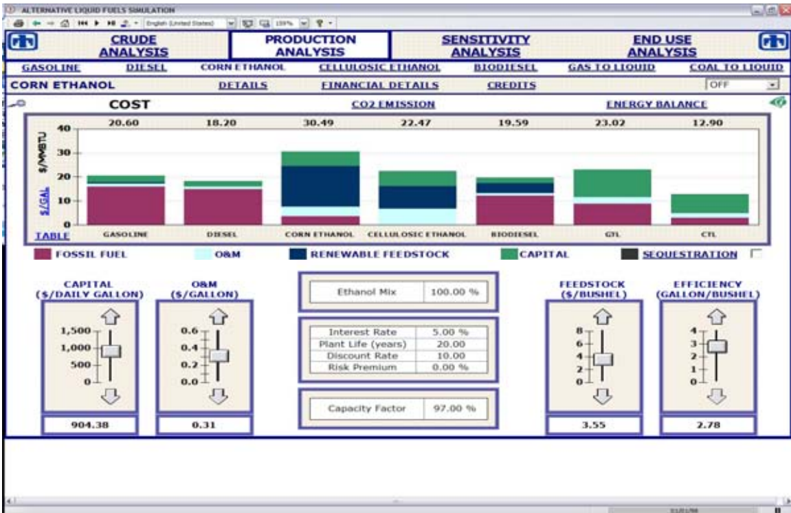
Figure 4. Representative AltSim Production Analysis Screen (corn ethanol) Showing Production Costs for all Fuels by $/MMBtu
