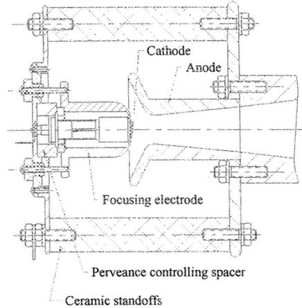
Figure 9: Schematic of the 20 A electron gun.
