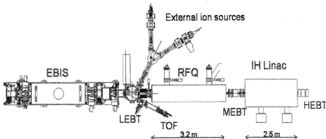
Figure 1: Layout of the EBIS Preinjector
