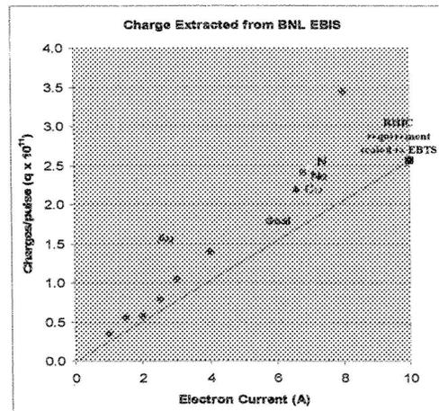
Figure 7: Ion yield vs. electron beam current, for various species
