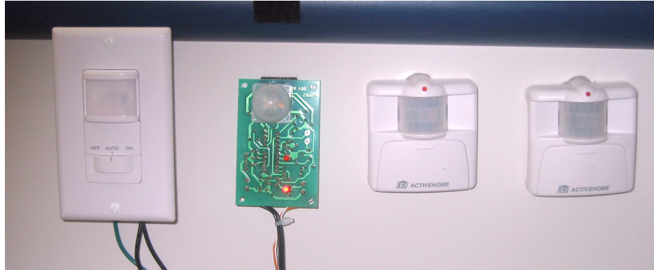
Figure 7-1. Sensor arrangement on one wall in the round-robin study
