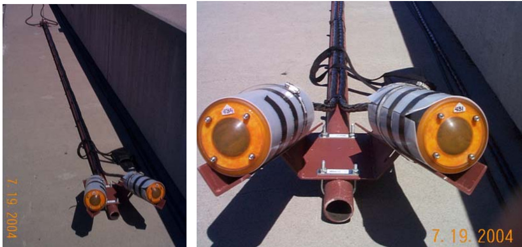
Figure 3.6. Wall-Mounted Splitbeam Transducers (pictured with acoustic lenses that were later removed; see discussion in Appendix B)
