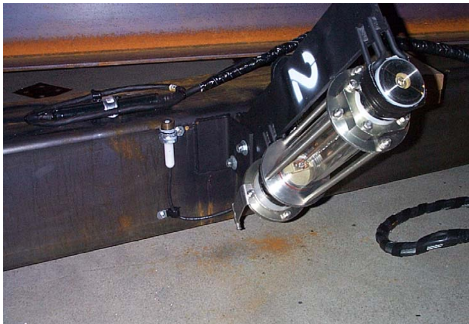
Figure 3.1. Aquatic Guidance Lighting Strobe Light Attached to Steel Beam for Deployment at Grand Coulee Dam in 2005
