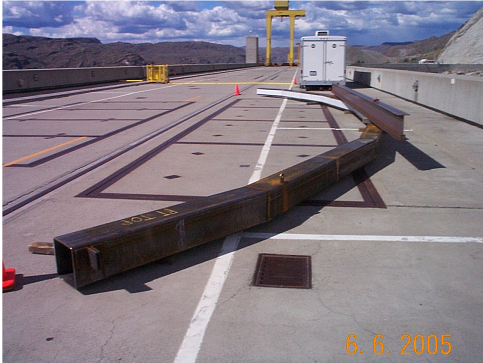
Figure 3.2. Strobe Light Assembly Bar (pictured prior to attaching strobe lights) with 11.3-m Lifting I-Beam on Top
