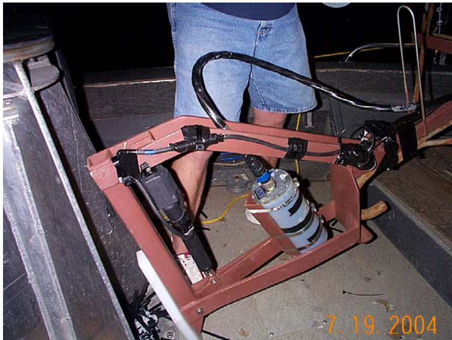
Figure 3.4. Splitbeam Transducer and Motorized Actuator on Trash-Rack Mount
