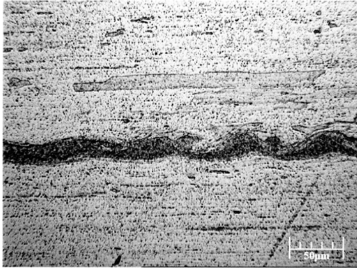
Fig. 34. Cross section of a joint in MA956 made by magnetic impulse welding. 30
