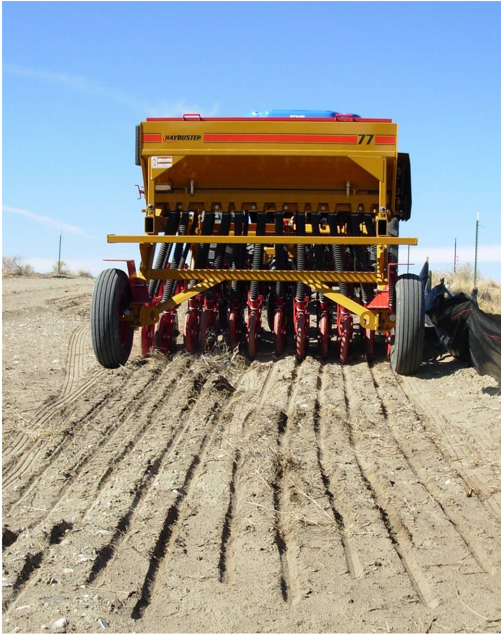
Figure 7. No-till Rangeland drill used to plant native seed at the Big Lost River Trenches.
