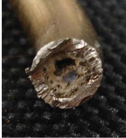
Figure 2-3. Photograph of mineral buildup in humidifier exit line.
