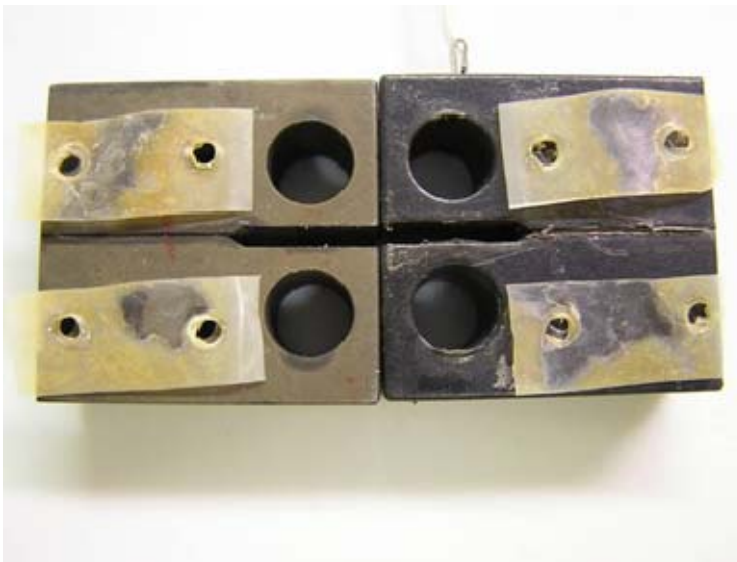
Figure III-3.26. Extensive crevice corrosion, due to delamination, in the periphery of the holes that were drilled to fasten the external cathodes
