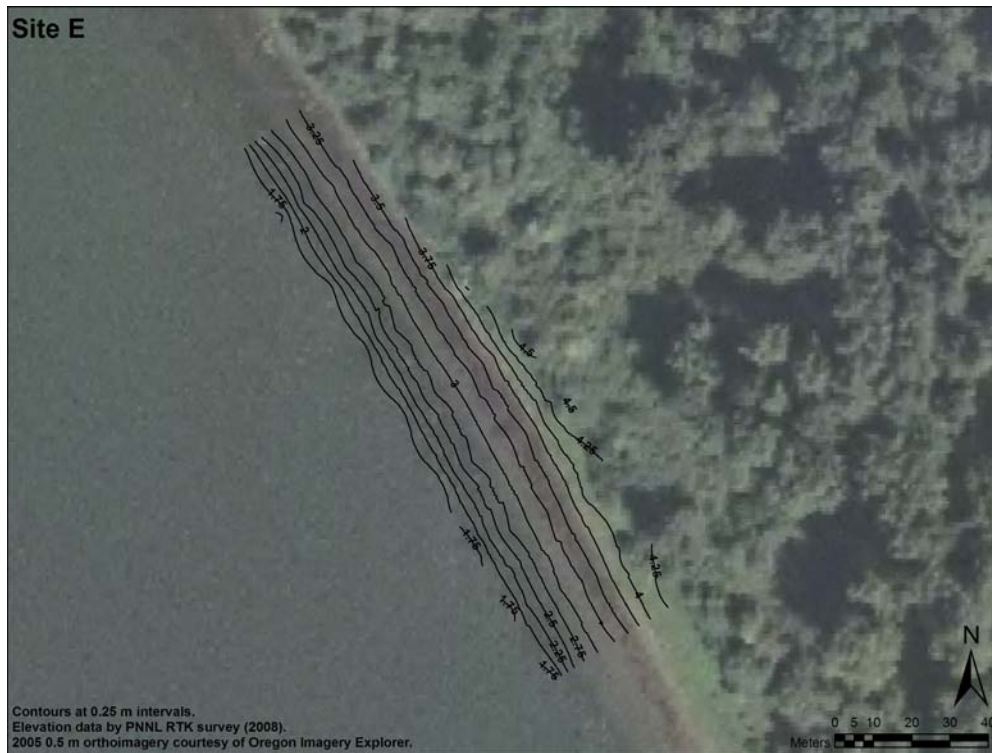
Figure B.5. Bathymetric Contours of the Beach Slope at Site E, Gary Island
