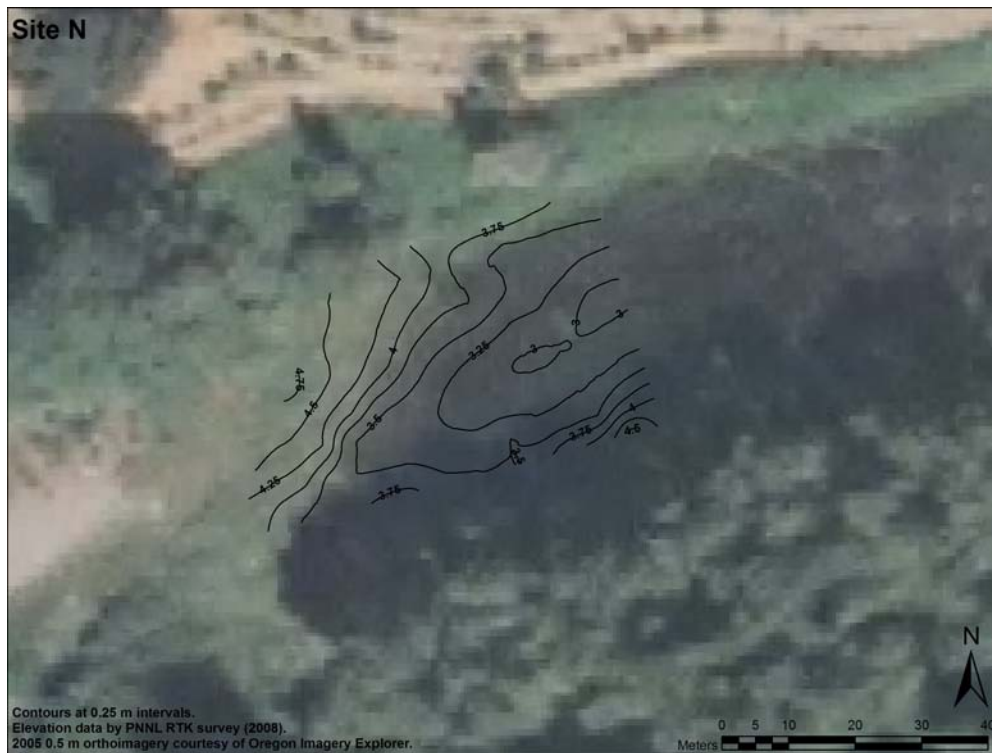
Figure B.8. Bathymetric Contours of the Beach Slope at Site N, the Blocked Channel in the Sandy River Delta
