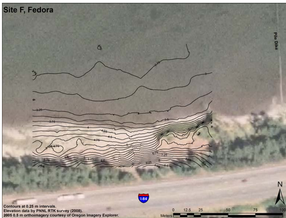
Figure B.6. Bathymetric Contours of the Beach Slope at Site F Adjacent to Highway 84 Upstream of Chatham Island
