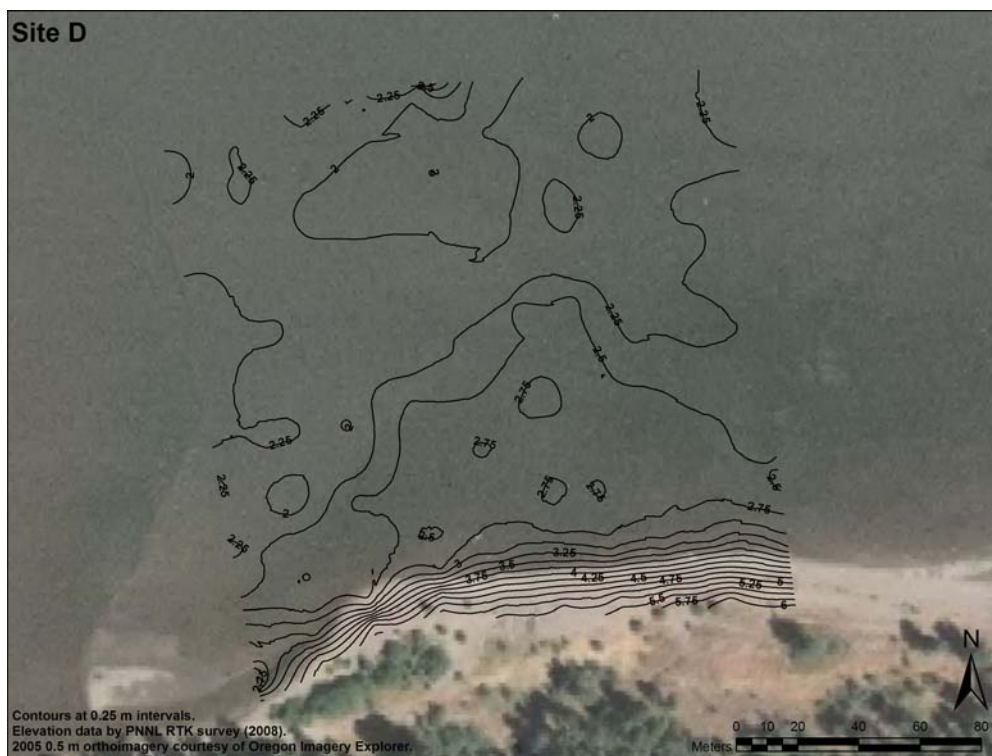
Figure B.4. Bathymetric Contours of the Beach Slope at Site D Adjacent to the Sandy River Confluence
