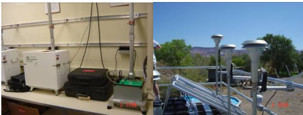
Figure 2. Photographs of PQ100 (green/gray box in left photo), PQ200 (white box in left photo) and their sampling inlets (right photo).
