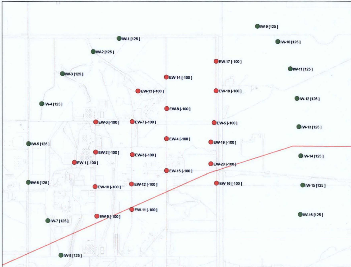
Fig. 1. Final groundwater extraction well and injection well network.
