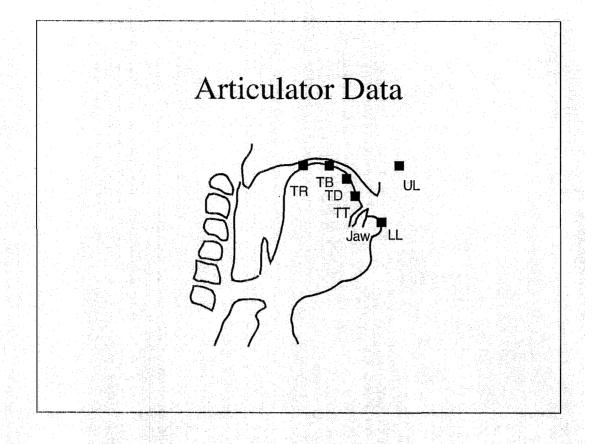
We also did an experiment with measured articulator positions and recorded speech. In this case we had a speaker produce vowel to vowel transitions and we recorded the positions of pellets glued to his tongue, jaw, and lips. The pellets are labelled ...
