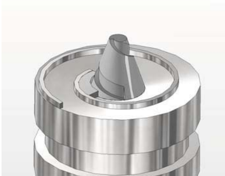
Figure 2: All tools were based on this scrolled pin and shoulder design. The tool with no scrolls was flat on the shoulder and the pin was smooth. The shoulder of the scrolled pin tool was also flat. The unscrolled pins were the dimensions of the pin above prior to cutting the scroll into it.
