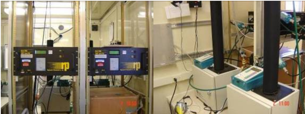
Figure 7. Left photograph: The front panels of PM 10 (right on the left photograph) and PM 2.5 (left on the left photograph) of TEOM. Right photograph: The DustTrak monitors (green) resting on top of the two TEOM measuring units.
