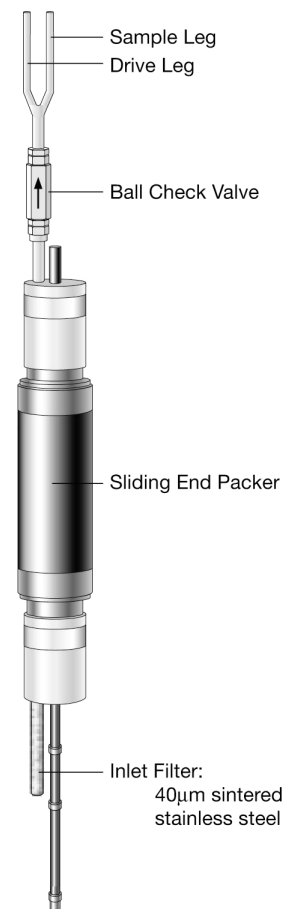
Figure 1. Schematic layout of the downhole equipment for deploying a U-tube geochemical sampler
