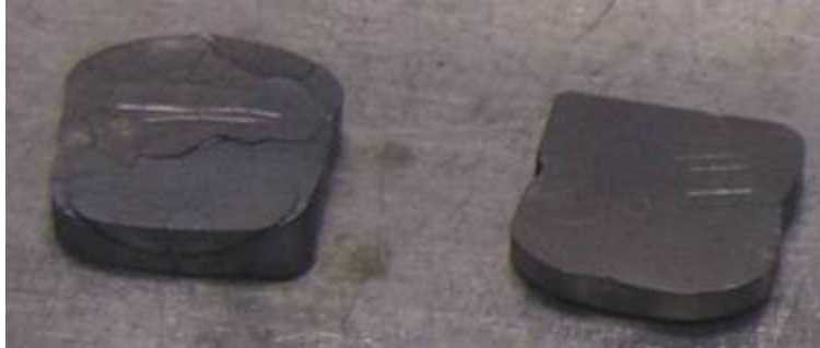
Figure 1. (UTh_4Zr_{10})H_{1.9} fuel disks fabricated at INL. The disk to the left has experienced cracking due to severe volume expansion.
