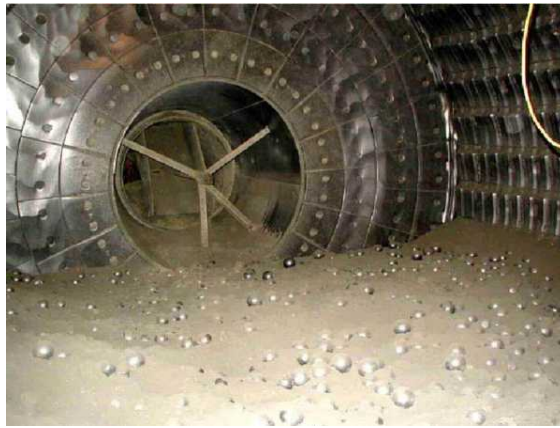
Steel grinding media interspersed with clinker in a cement mill, image courtesy Castle Cement, taken from http://www.understanding-cement.com/mill.html
