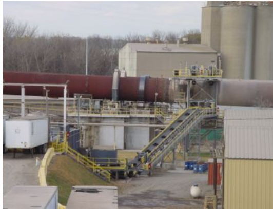
(a) Cement kiln using used tires in the kiln, image taken from Wikipedia at http://en.wikipedia.org/wiki/Portland_cement . (b) Chipped tires as a substitute fuel at the Cemex Rugby cement works in Warwickshire, U.K., image taken from http://www.letsrecycle.com/do/ecco.py/view_item?listid=37&listcatid=317&listitemid=9464
