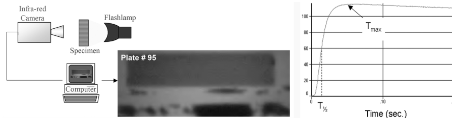
Fig. 4. Simple schematic of the through-thickness flash thermography technique illustrating qualitative analysis capability (left); Example thermal diffusivity profile obtained from through-thickness flash thermography illustrating quantitative analysis capability (right).
