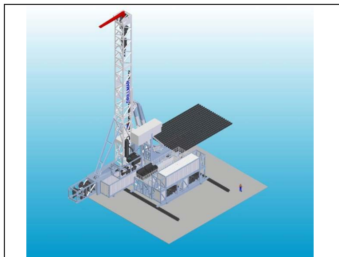
Figure 32. Huisman LOC250 well pad (platform) layout.
