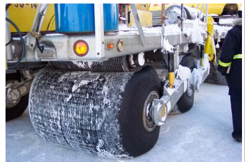
Figure 20. Close-up of Rolligon low-pressure tires.
