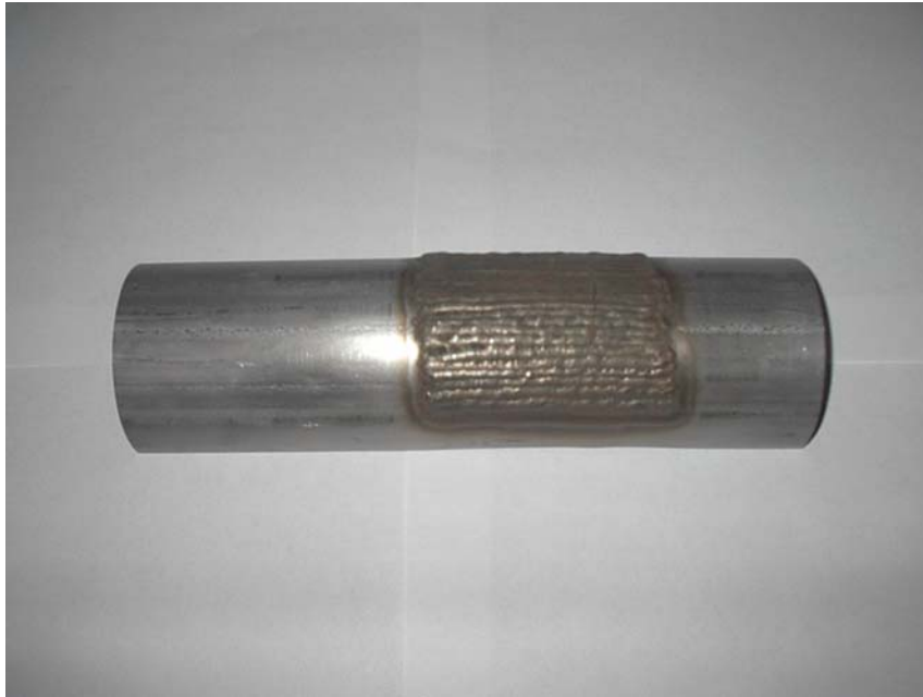
Figure 5. Overview of Fe 3 Al coated on half-circle-shaped 304 stainless steel
