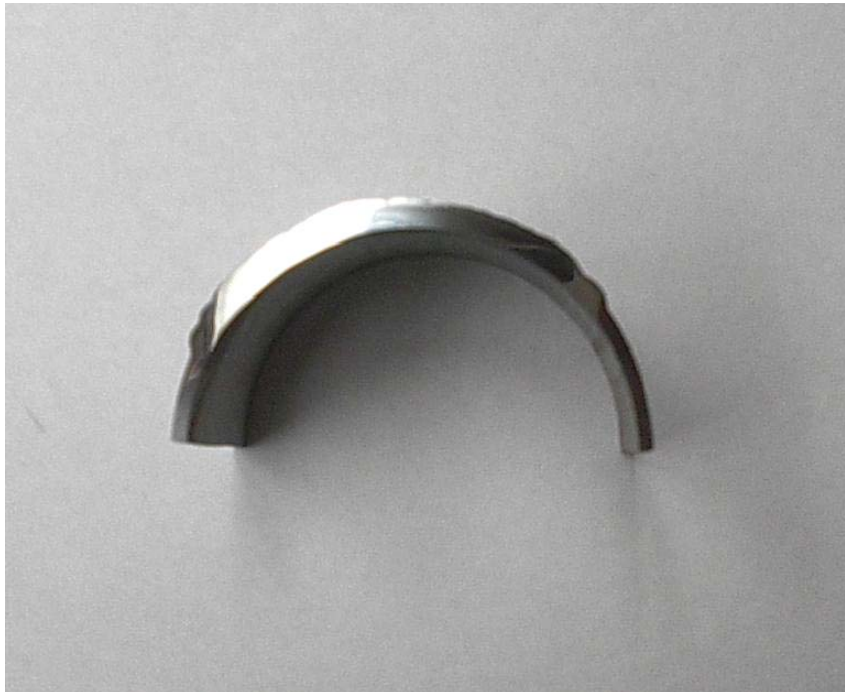
Figure 6. Cross-sectional view of Fe 3 Al coated on half-circle-shaped 304 stainless steel
