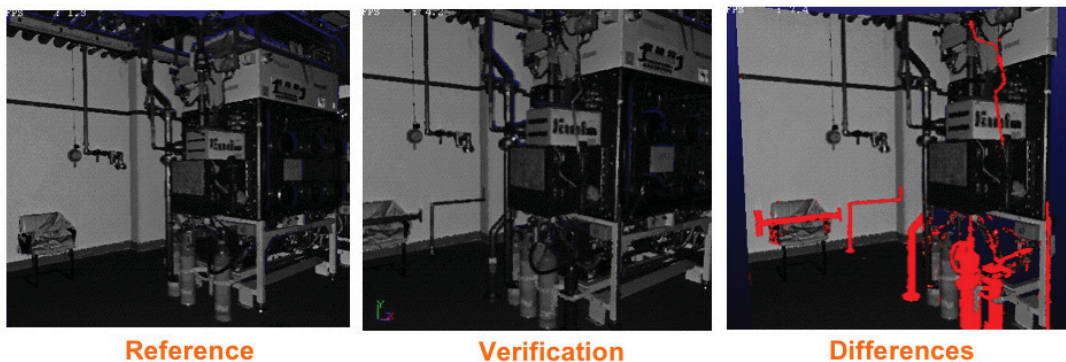
Figure 2: 3DLR Automated Change Scene Detection Feature. (Areas changed prior to re-verification are automatically highlighted in red.)
