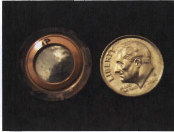
Figure 1. A typical composite membrane disc sealed between two Cu VCR gaskets (Ni gaskets are normally used). This 0.37-mm thick V-6Ni-5Co membrane (coated with 100 nm Pd per side) was tested for 170 h at 450°C. 48
