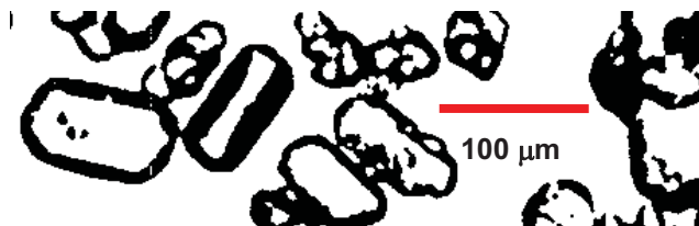
Fig. 10. (U,Pu)O 2 crystals produced by AUPuC fabrication
