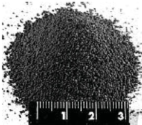
Fig. 16. Calcined granules of MOX powder produced by the Granat process. (scale in cm.)
