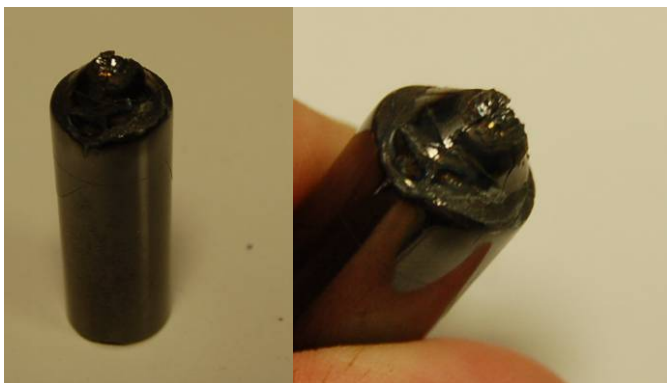
Fig 5 & 6: Warped crucibles after AlSb melting
