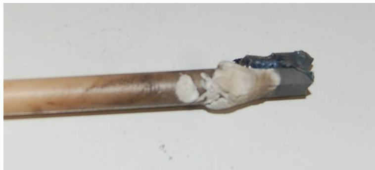
Fig 8: AlSb that melted on itself
