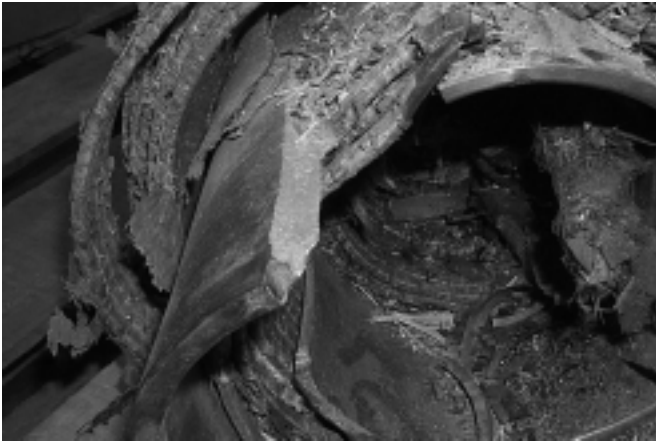
Fig. 3: Photograph of coil 4 fracture shear lip.
