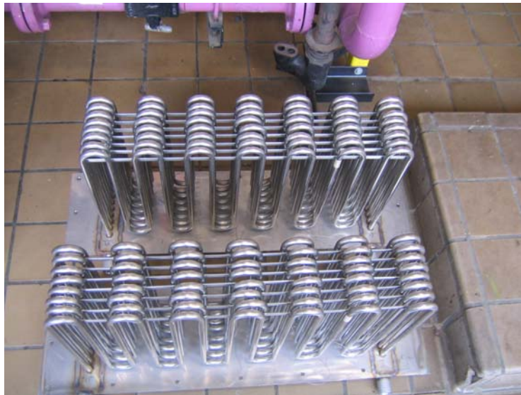
Figure 2-3: Photograph of Two Bare Tube Heat Exchanger Bundles.
