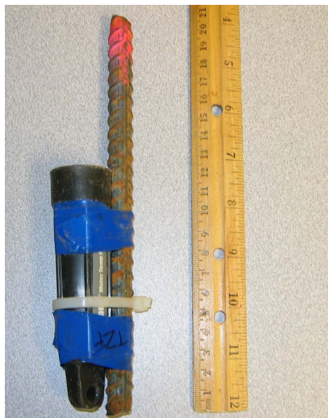
Figure 2.5. Onset Sensor Attached to Rebar Stake
