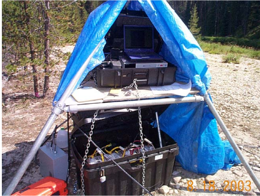
Figure 2.8. Surface Components of the Acoustic Camera and Optical Camera System
