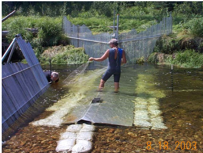
Figure 2.7. Secesh River Counting Station. The direction of flow is from right to left. (Note: artificial substrate should be installed with the steep side toward the right or upstream.)
