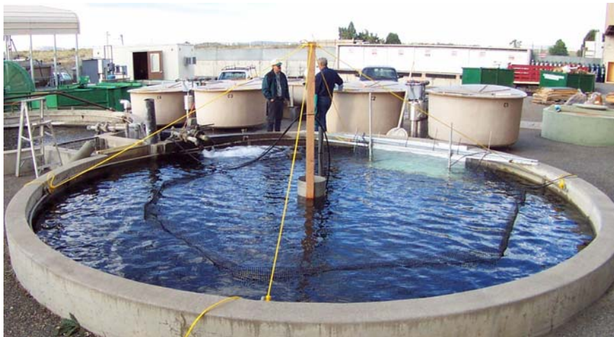
Figure 2.11. Circular Concrete Tank (6.1 m [20 ft] in diameter by 0.7 m [2.3 ft] deep) Used for Laboratory Validation Tests at the Pacific Northwest National Laboratory Fish Facility
