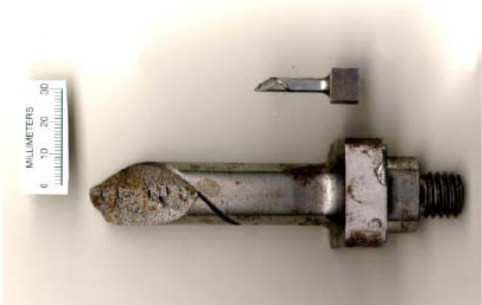
Figure 8 SNTT Specimen miniaturization for A533B steel.
