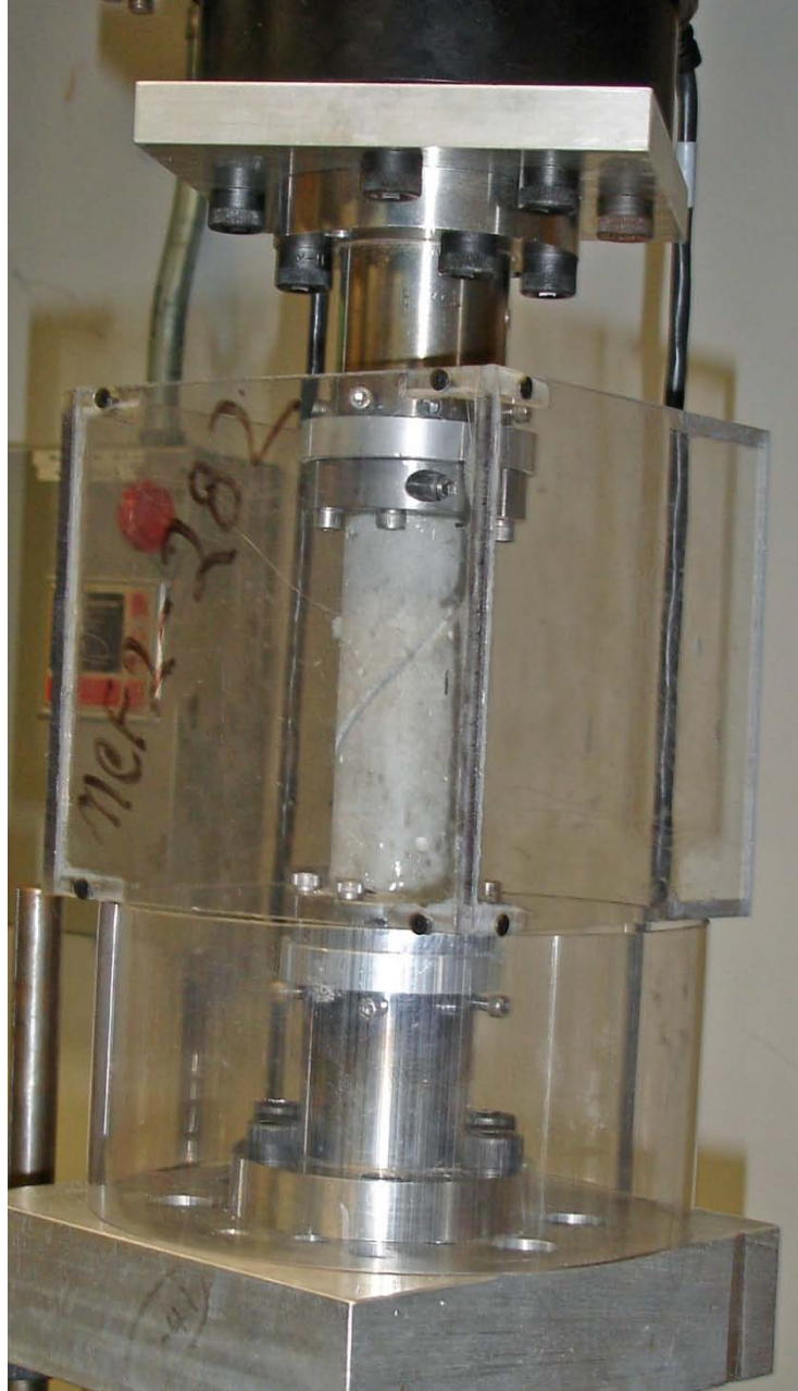
Figure 20 SNTT mortar testing set-up with the protective shield.
