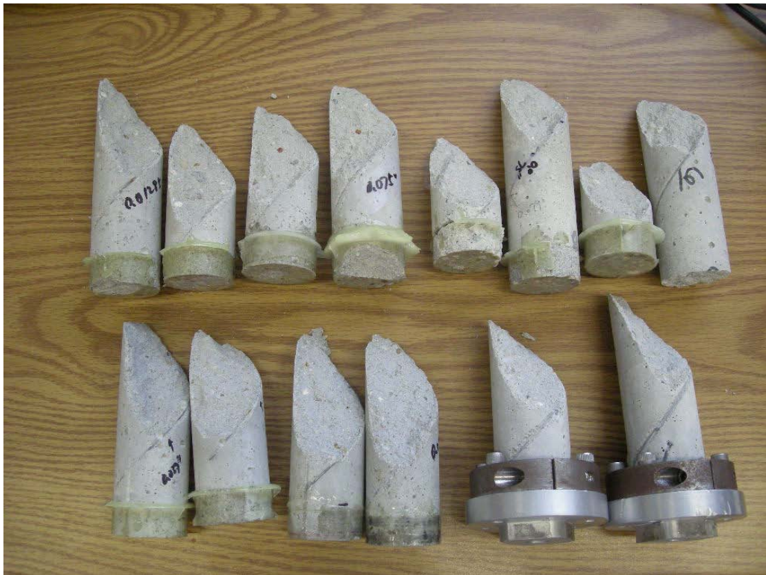
Figure 21 Fractured SNTT mortar sample shows classical tension brittle fracture characteristic.
