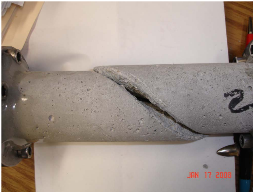
Figure 19 SNTT test assembly and fractured SNTT sample.
