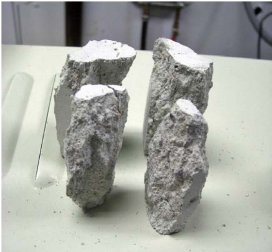
Figure 13 Compression fractured samples, w/ Teflon insert at loading boundary. r.h.s. shows typical fracture columns.
