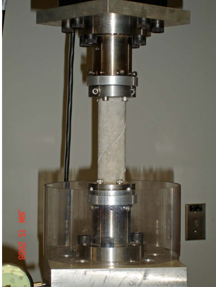
Figure 4 SNTT mortar test set-up.
