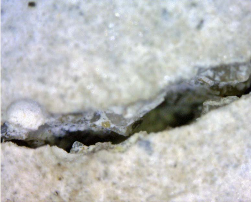
Figure 15 Fracture surface along the 45° spiral groove.
