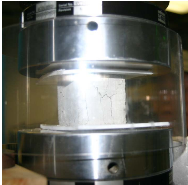
Figure 13 Compression fractured samples, w/ Teflon insert at loading boundary. r.h.s. shows typical fracture columns.
