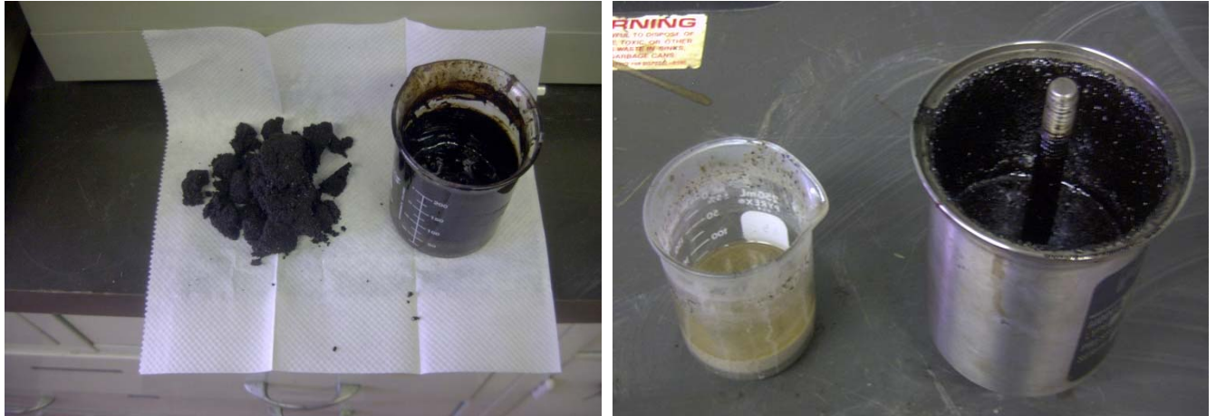
Figure 7. Left picture: Asphalt Ridge oil sands, Utah, containing 12 \pm 1.7\% bitumen by weight. Right picture: Depleted and settled oil sands (beaker) and extracted, separated bitumen (canister) (Conditions: 85^\circ\text{C} , 100 psi, 20 cycles).
