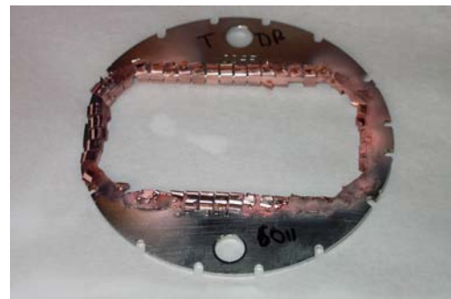
Figure 2: Rf seal damaged by beam-induced heating.
