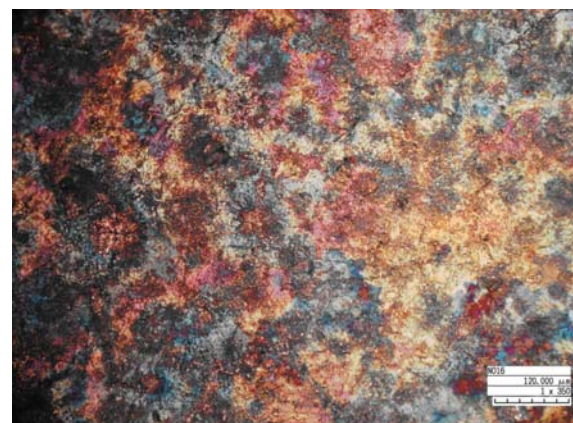
Figure 7: Picture of copper electrode surface after the breakdown experiments. Blue and red discolorations are copper oxides and the white areas correspond to sulphur. The total width of the picture is about 1 mm.
