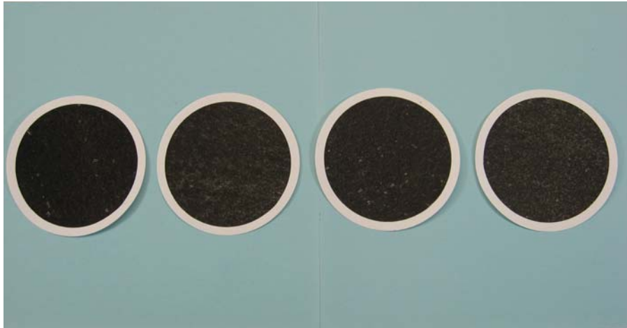
Figure 5.40: BP-15 with 40% energy equivalent DME: 2°, 3°, 5°, 7° BTDC (left to right)
