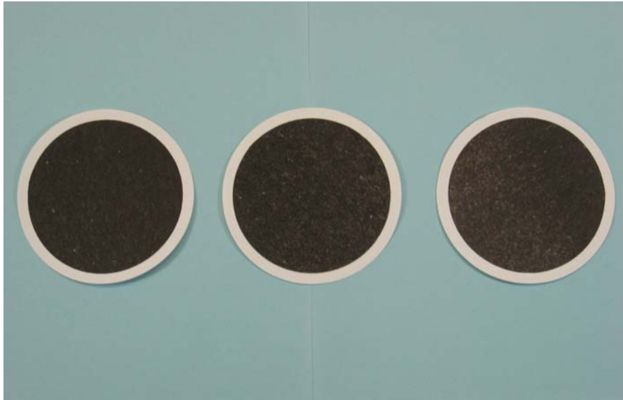
Figure 5.39: BP-15 with 25% energy equivalent DME: 1°, 3°, 7° BTDC (left to right)
