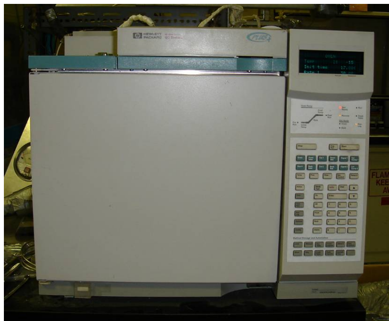
Figure 5: Gas Chromatograph (GC) for HC Speciation of Exhaust Gas
