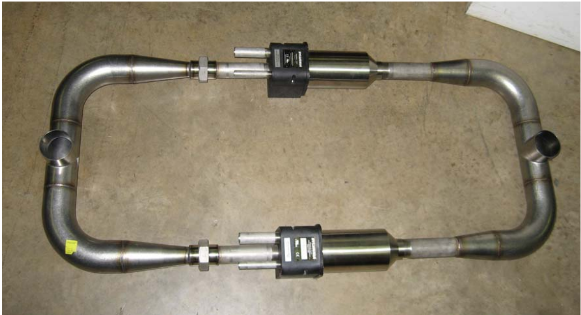
Figure 5.10: Layout of intake air heating system before installation on the DDC 2.5L engine stand
