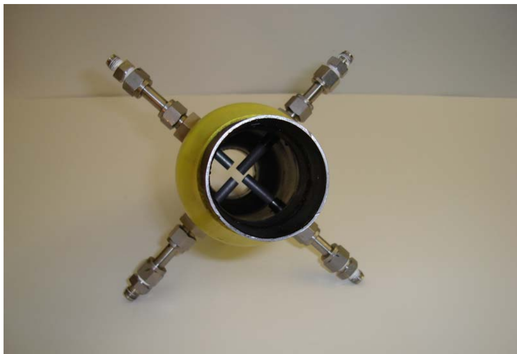
Figure 5.1: Custom intake air manifold aspiration system
