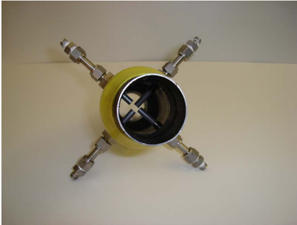
Figure 3.4: Custom intake air manifold aspiration system.
