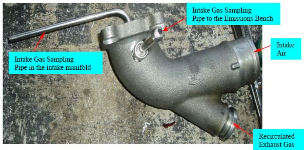
Figure 3.2: Instrumented air intake/EGR Y-pipe.
