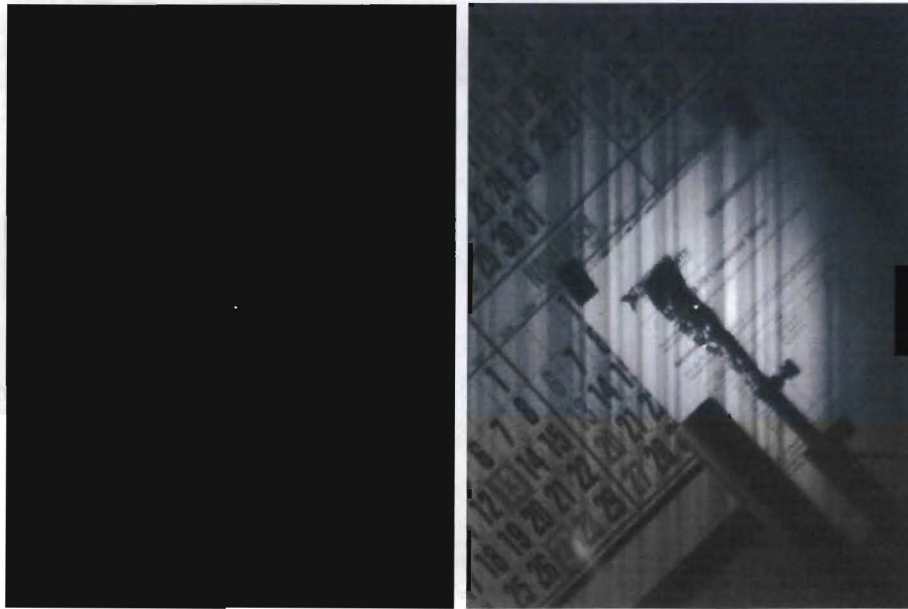
Figure 9. Comparison of signal levels obtained for a single slit spectral imager, as simulated using the micro-mirror array (left), and for an 83-band Hadamard transform spectral imager implemented on the micro-mirror array (right). Light levels, integration times, spectral bin widths, and all other parameters are identical for two cases.
