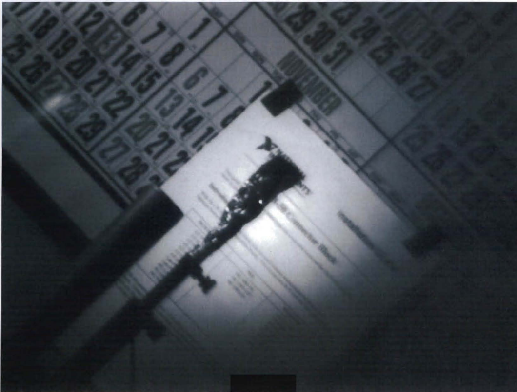
Figure 7. Broad-band image of a typical test scene obtained with the prototype micro-mirror instrument. The scene consists of a wall calendar illuminated by both a mercury-vapor lamp, visible near center, and an incandescent lamp located off the left side of the image. The Hg lamp provides a sharp line spectrum consisting of four lines in the instrument's spectral range. The shortest wavelength of these lines is strongly absorbed by the calendar's glossy coating. A sheet of uncoated white paper, which reflects all four Hg lines, is also included in the scene. The 45-degree rotation of the scene follows from the orientation of the micro-mirror array, which in turn derives from the along-diagonal tilt direction of the micro-mirrors.
