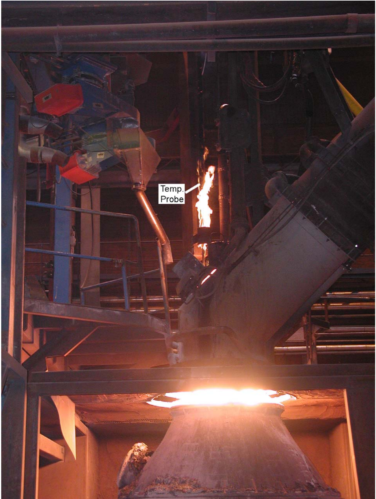
Figure 12 Temperature probe removal during decarburization for Universal Converter
