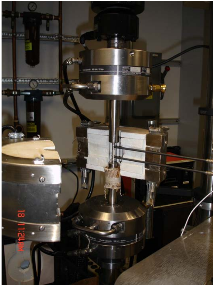
Figure 5-3 Close-up of environmental chamber and the extensometer, which is part of integrated test controls system for measurement deformation.
