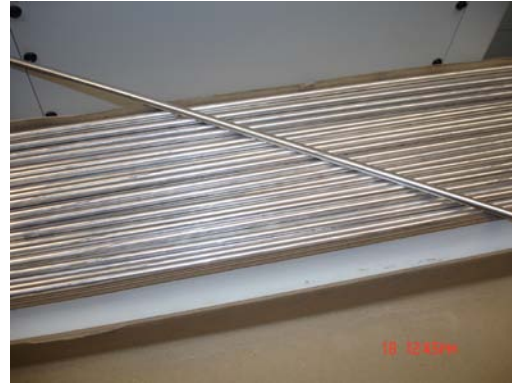
Figure 5-12 Second order of 1350-H19 rod with #1 AWG size, at 0.28 inch diameter.
