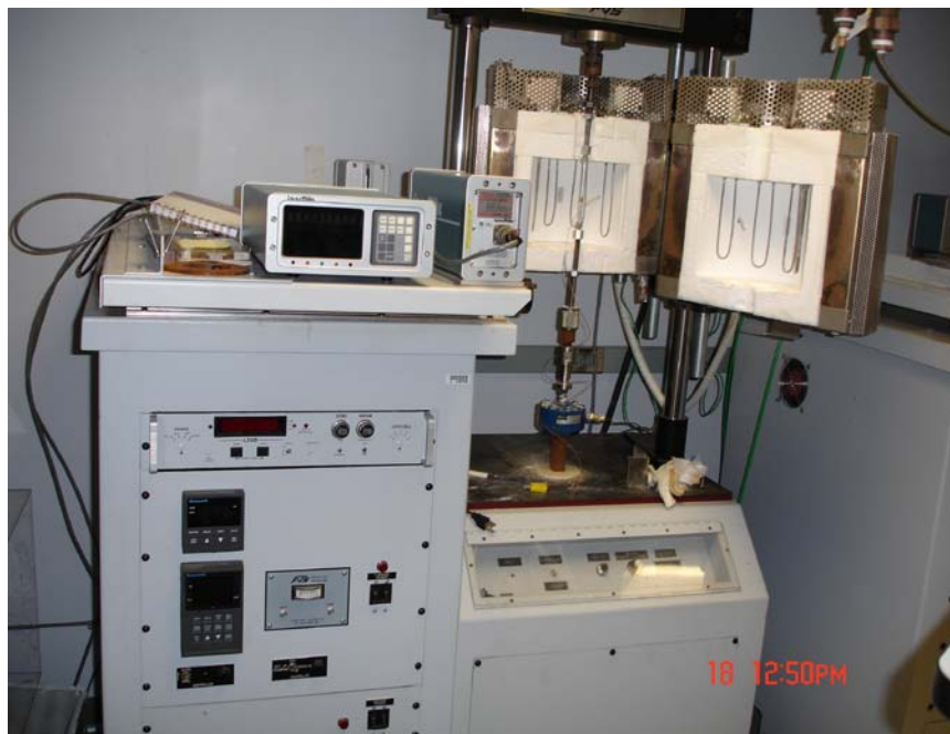
Figure 5-9 A close-up of one ATS creep test machine, with a visual of the interior of the environmental chamber. The left tall cabinet is the furnace and temperature control system and the right cabinet is the load control system.
