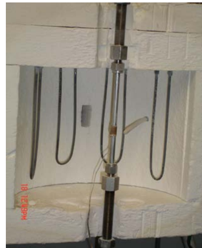
Figure 5-14 The end-grip design for pilot tensile testing.
