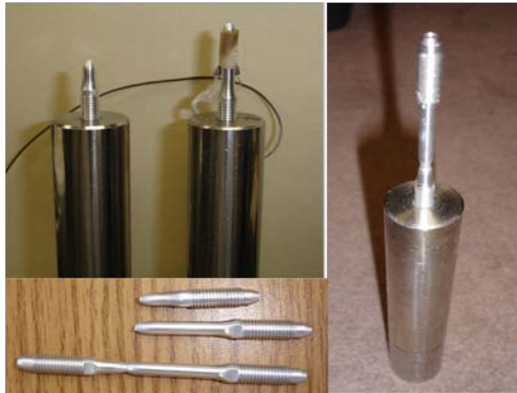
Figure 5-20 Fractured tensile specimens and end-grip.
