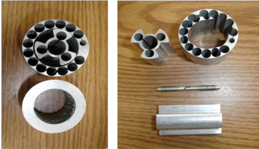
Figure 5-26 Tensile and fatigue samples for 3003-H183 and 6061-T6 materials were machined directly from the baseline splice sleeve and the associated core-grip.
