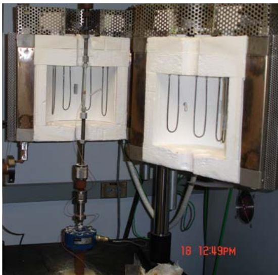
Figure 5-13 Pilot tensile testing set-up in an ATS creep machine with the associated loading train.
