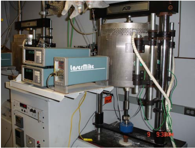
Fig. C10 Creep test set-up, including environmental chamber, load frame & load controller, Laser Mike, and furnace control.
