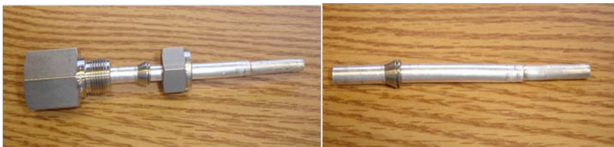
Figure 5-16 (Left) The typical slippage failure of 1350-H19 rods at grip-end during pilot tensile testing. The reduced section at the grip-end is due to a pipe fitting ring bitten into the testing sample. (Right) Details of a tensile sample failed at grip-end, and the intact side with the pipe fitting ring.
