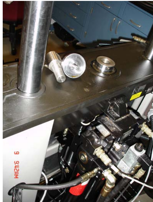
Fig. C14 The hydraulic oil leaking from actuator of MTS 810 tester.
