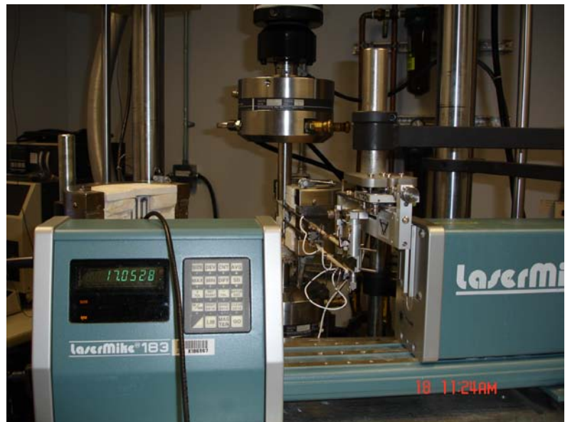
Figure 5-4 Close-up of the Laser Mike and the calibration band attached at the end of extensometer for strain measurement.
