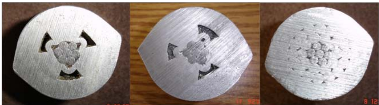
Figure 6-4 Typical cross-sections of ACSR Drake SSC system: (left, middle) core-grip section, and (right) conductor section.
