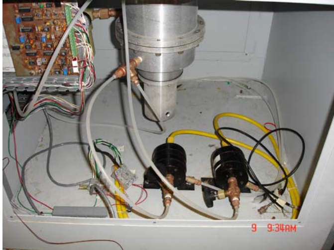
Fig. C13 ATS creep testing lower chamber that contains pneumatic pumps and system controller.
