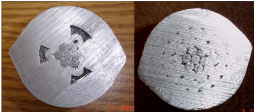
Figure 6-21 Cross-sections of the irradiated SSC samples: (left) core-grip section, (right) conductor section.
