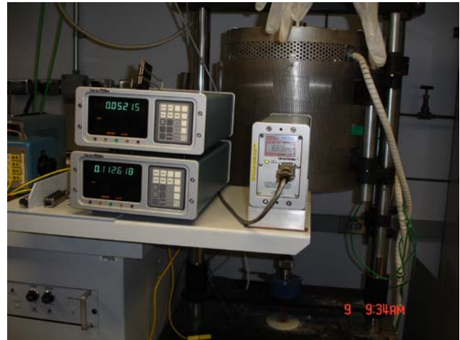
Fig. C11 Detailed view of Laser Mike set-up and its alignment with the window of furnace.
