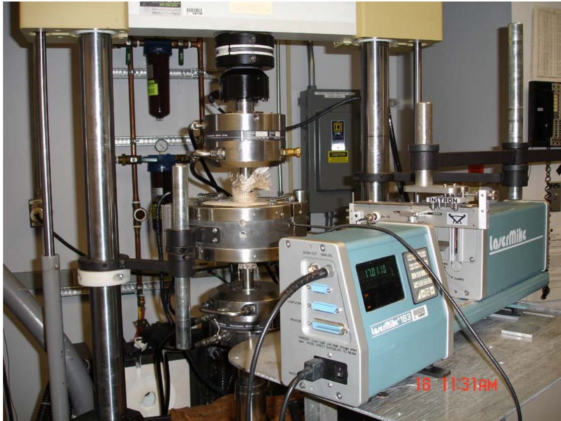
Figure 5-5 High temperature tensile test with the associated deformation control set-up.
