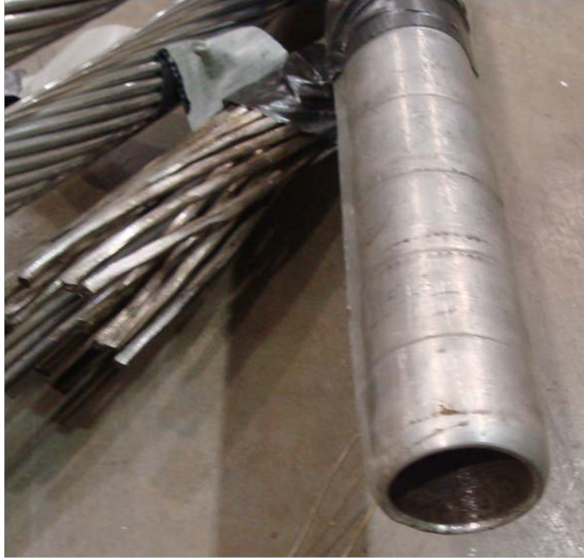
Figure 8-5 SSC fitting sleeve and the Drake conductor after the pull-out test.
