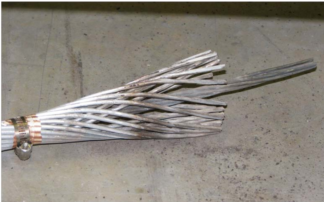
Figure 8-4 Drake conductor after SSC fitting pull-out test.
