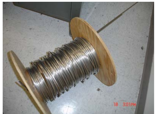
Figure 5-11 First order of 1350 aluminum shipped with an 8 inch diameter barrel.
