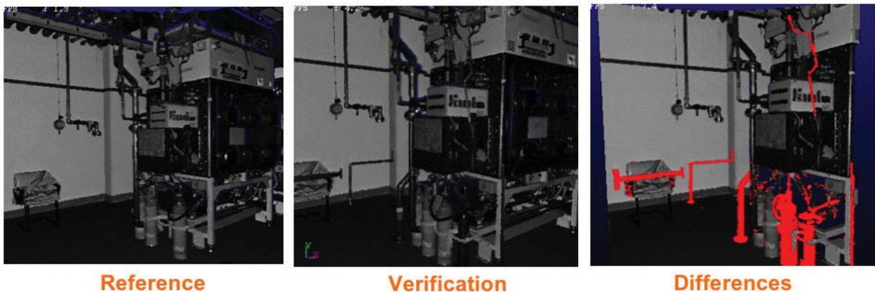
Figure 1. 3DLR Automated Change Scene Detection Feature. The 3DLR has been designed to compare two images and highlight the differences. [Ref. 7]
