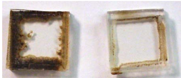
Figure 12. Photograph of ionomer sample after exposure to 42 UV suns.
