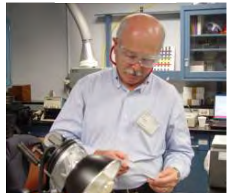
Fig. 6-2. Todd Cleaver, Ford Motor Co., examining a spot weld specimen.
