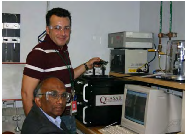
Fig. 3-15. Professor Sooryakumar (Ohio State University) and MCAUC's Miladin Radovic using resonant ultrasound spectroscopy to determine the elastic properties of TiC-particulate-reinforced titanium matrix composites.
