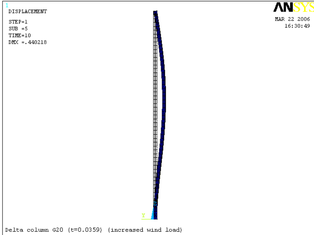
Figure 5.11 Deformation of the Delta-shape column with 20 Gage (unit: inches)
