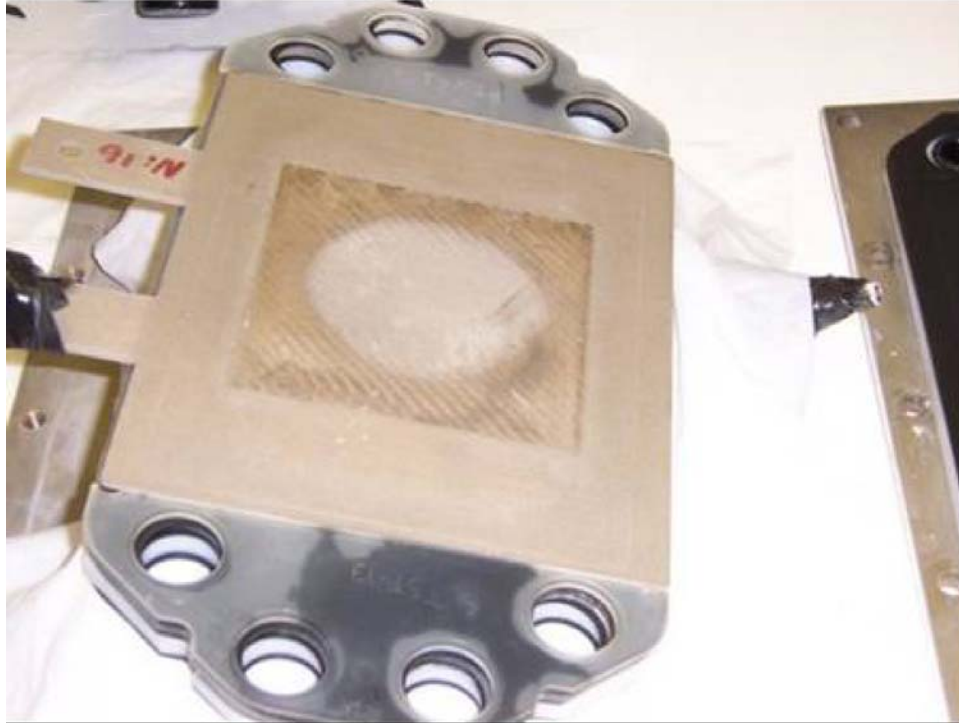
Figure A.13. Back Side of Nickel Electrode. Interesting shadow impression of membrane. Discoloration surrounding membrane shadow.
