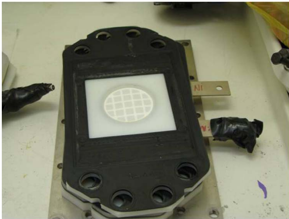
Figure A.8. LANS Membrane on the Anode (Kovar™ Electrode) Side. No irregular observations.
