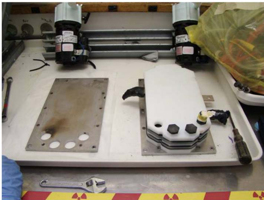
Figure A.2. Discoloration on the Backside of the Support Plate at the Catholyte Inlet Was Observed and Cause Unknown
