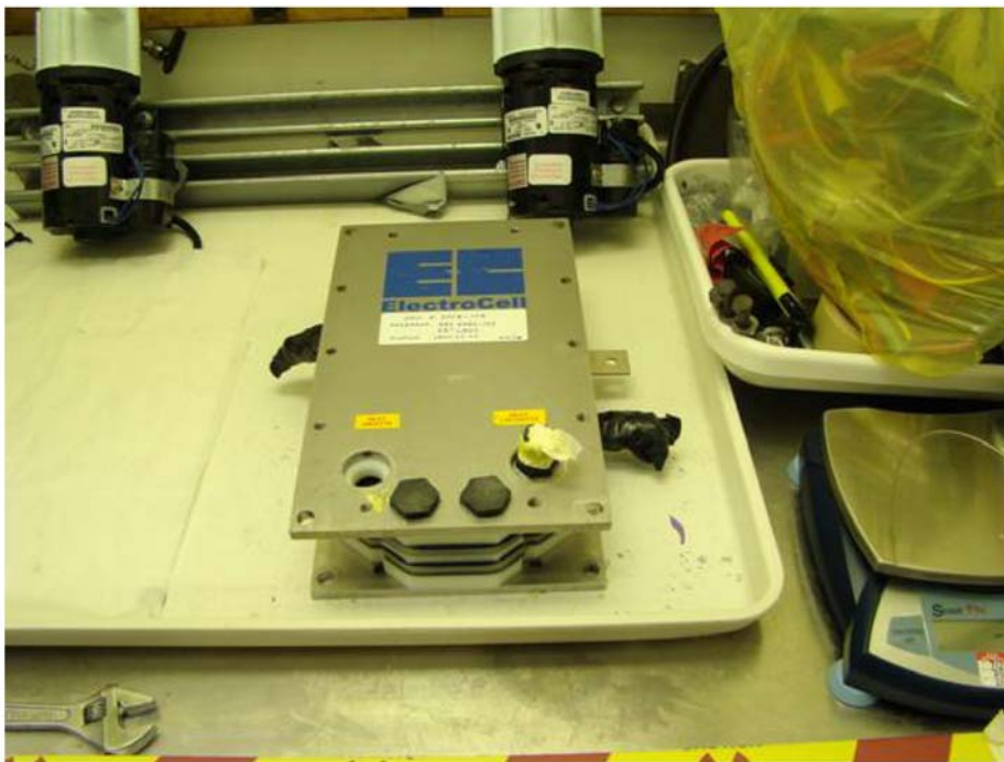
Figure A.1. Cell Bolts Removed
