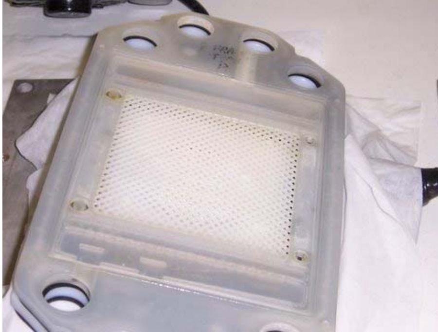
Figure A.11. Nickel Electrode Side of Flow Promoter. No irregular observations.
