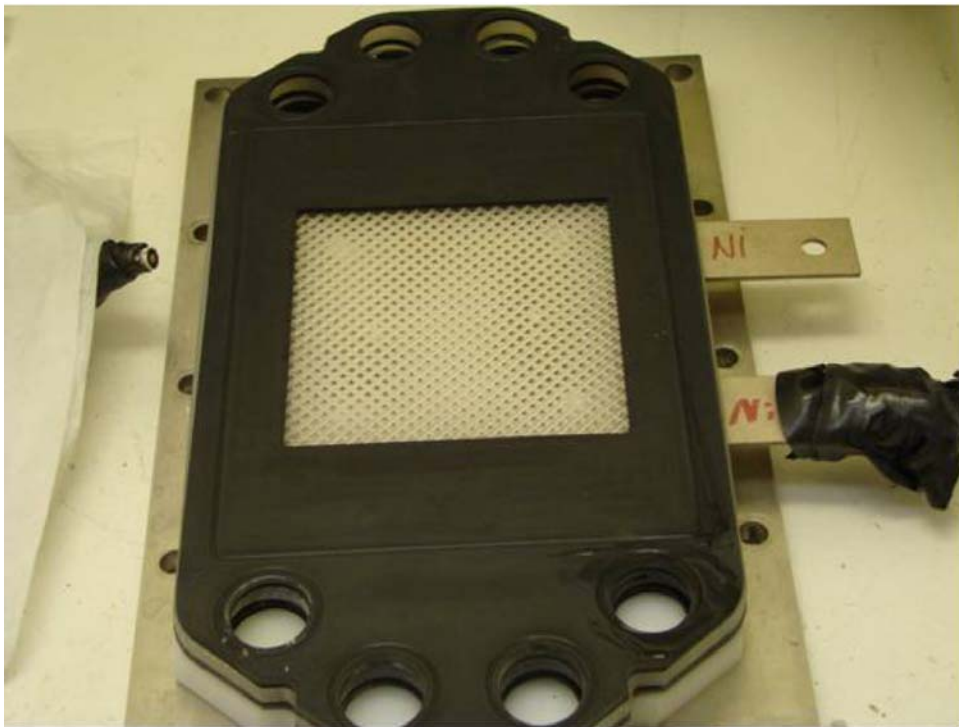
Figure A.10. Membrane Side of the Cathode Side of Flow Promoter. No irregular observations.
