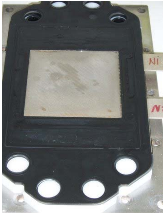
Figure A.12. Membrane Side of the Nickel (Cathode) Electrode. Relatively uniform coloration.
