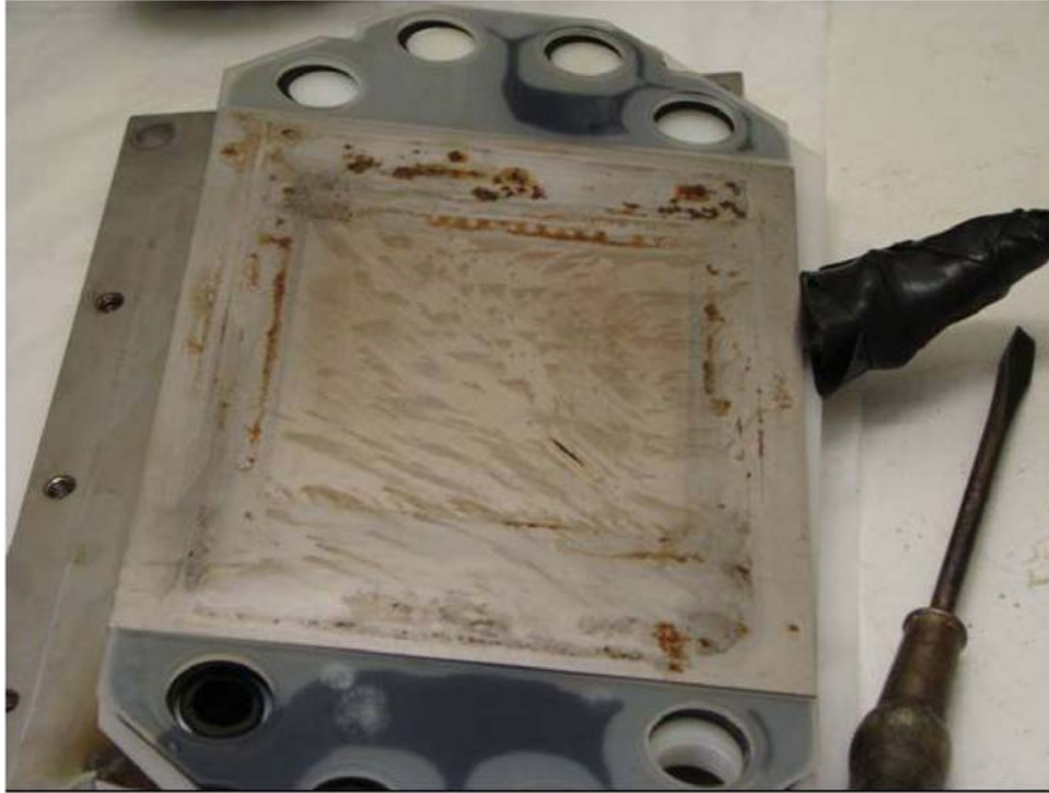
Figure A.5. Membrane Side of the Kovar™ Electrode. Discoloration Appears to Be Corrosion Byproducts
