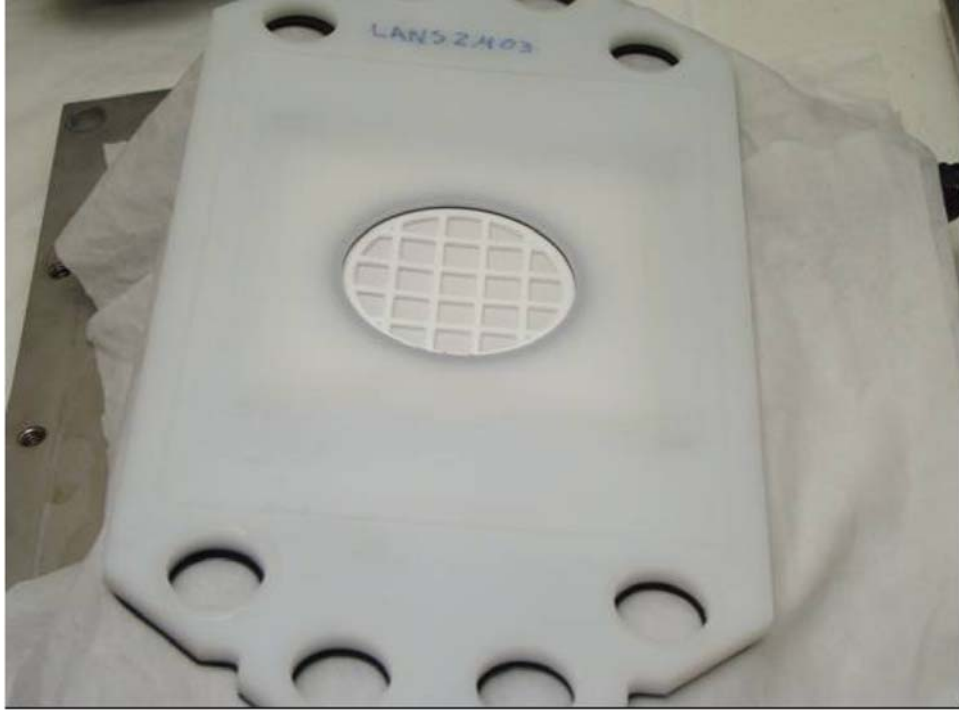
Figure A.9. LANS Membrane on the Cathode (Nickel Electrode) Side. No irregular observations.
