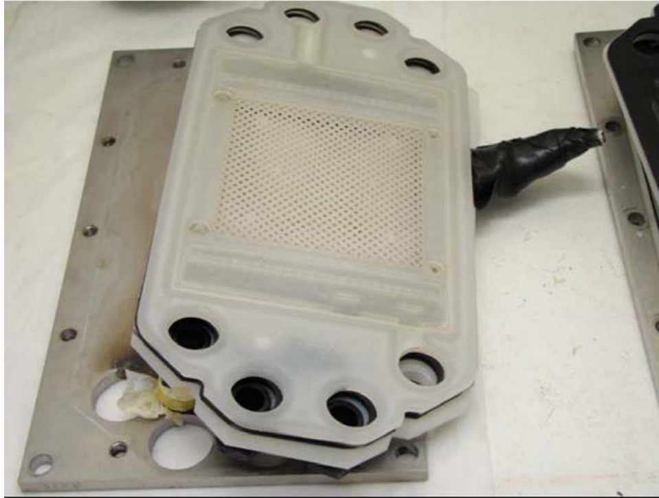
Figure A.7. Membrane Side of the Flow Promoter. No solids observed on the flow promoter.
