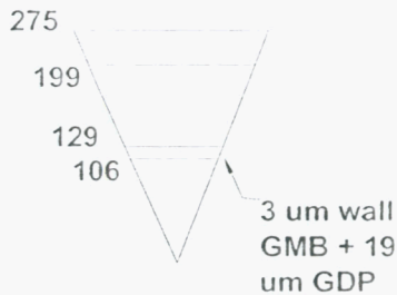
Type A thick ablator imaging capsule
