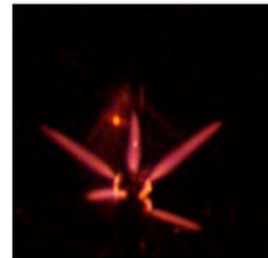
100kpa neon with small amount of air, 14khz
