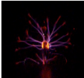
60kpa neon with trace xenon 30 khz
