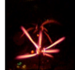
100kpa neon with small amount of air, 66khz
