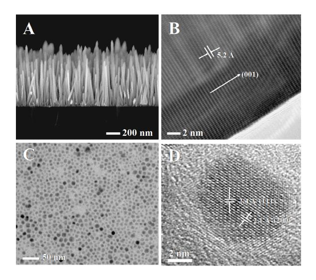
**Figure 1.** A) Cross-sectional SEM image of ZnO nanowire array used in solar cells, prior to  $Cu_2O$  addition. B) High-resolution TEM image of an individual ZnO nanowire. C) Low r
