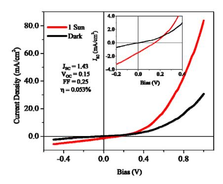
**Figure 7.** J-V curves of a  $ZnO/TiO_2/Cu_2O$  solar cell in darkness and under 1 Sun illumination. The  $Cu_2O$  film was annealed at  $300^{\circ}C$  under 500 mTorr oxygen. The ZnO NWs are 500 nm in length, the  $TiO_2$  coating layer is 10 nm thick, and the  $Cu_2O$  film thickness is 800 nm.
