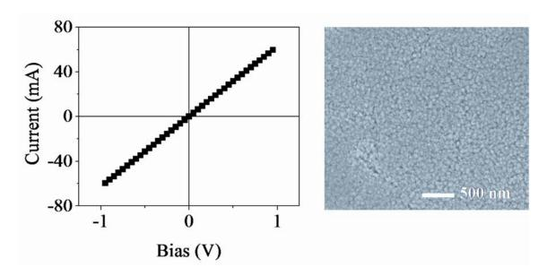
**Figure 6.** J-V Curve of a ZnO/Cu<sub>2</sub>O solar cell with no interceding  $TiO_2$  layer, and corresponding top-down SEM image.
