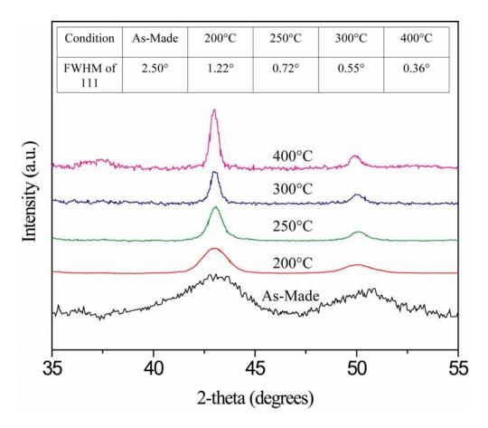
**Figure 5.** XRD patterns of  $Cu_2O$  NPs films on glass, annealed at the noted temperatures under 500 mTorr oxygen (Total pressure = 5 Torr). The patterns are vertically offset for clarity, and the accompanying table lists the measured FWHM values for the 111 peak at the different annealing temperatures.
