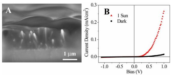
**Figure 2.** A) Cross-section SEM of a completed ZnO/Cu<sub>2</sub>O solar cell, with no Cu<sub>2</sub>O annealing performed. B) The corresponding J-V curve in darkness and under 1 Sun illumination.
