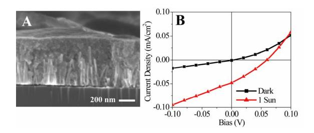
**Figure 4.** A) Cross-section SEM of a completed  $ZnO/Cu_2O$  solar cell, with the cell annealed at  $200^{\circ}C$  after each application of  $Cu_2O$  NPs. B) The corresponding J-V curve in darkness and under AM 1.5 and 1 Sun illumination.
