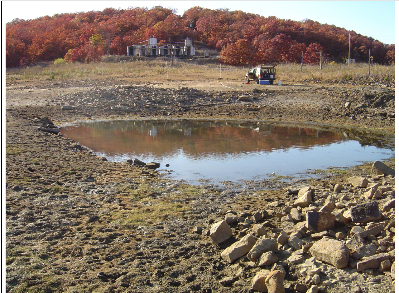
Figure 6. The oil production site during drought conditions that occurred over the summer and fall of 2006. The pool in the center of the photo is the submerged brine pit which is under 3-4 m of water when lake levels are normal. The white rope along the ground in the upper right side of the photo (left side of vehicle) is a transect line normally used by divers to deploy in situ exposure chambers and collect field samples.
