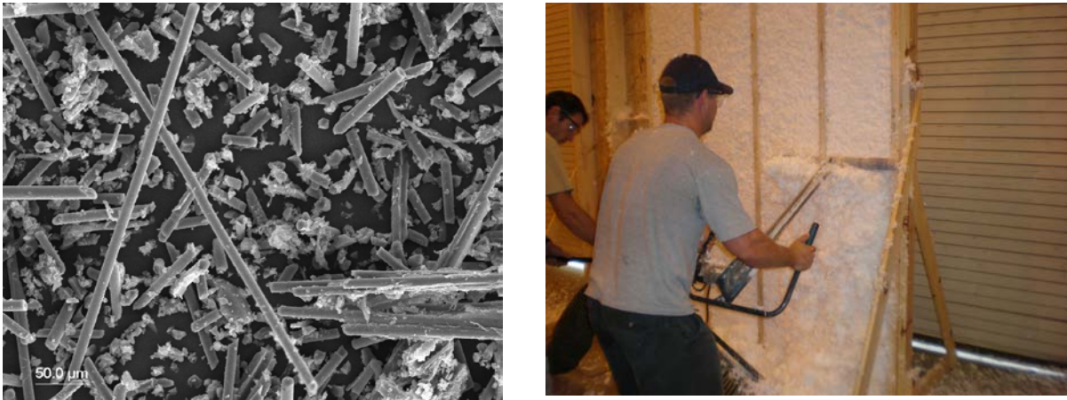
Fig. 1. Microscopic view of a complex network of glass fibers within the blown insulation, and installation of the blown fiber glass into the test wall.
